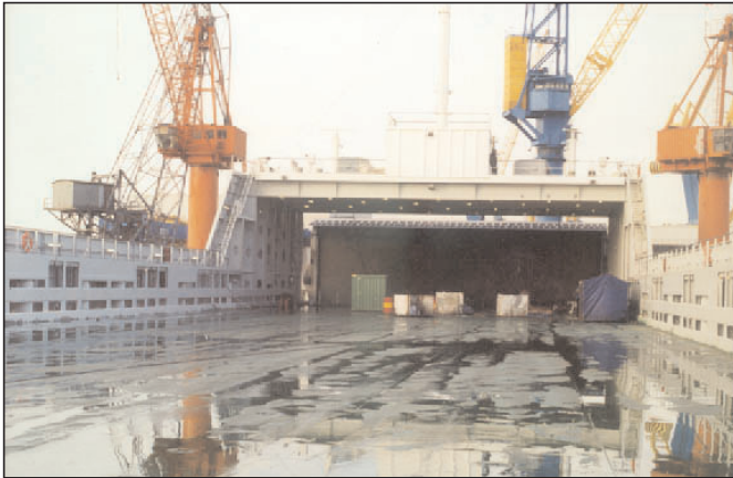
Left: An ideal IPSI ship for containers and trailers would feature a series of kerbs so that automated guided vehicles could place unitised cargoes exactly into position; on the Spaarneborg only the strong bulwark barriers seen here will be used, since SECUs will be block-stowed. Right: In the main and tanktop decks, a series of centreline barriers is fitted. Fixed Hamworthy KSE ramps port and starboard lead to the lower level; their lower ends have a hinged section, which stows flush and horizontal to gain four extra SECU positions.
