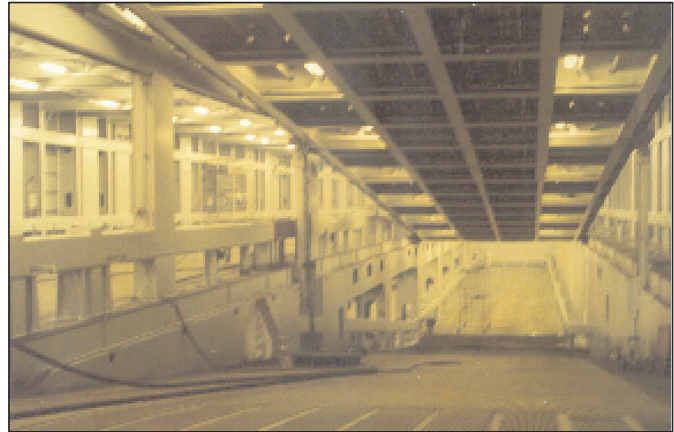
Left: An ideal IPSI ship for containers and trailers would feature a series of kerbs so that automated guided vehicles could place unitised cargoes exactly into position; on the Spaarneborg only the strong bulwark barriers seen here will be used, since SECUs will be block-stowed. Right: In the main and tanktop decks, a series of centreline barriers is fitted. Fixed Hamworthy KSE ramps port and starboard lead to the lower level; their lower ends have a hinged section, which stows flush and horizontal to gain four extra SECU positions.
