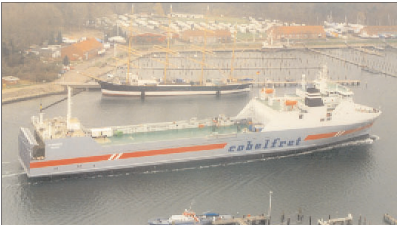
Spaarneborg negotiating the river Trave. This interesting 12,500dwt ro-ro vessel and her two sisters will pioneer a new intermodal system of transporting paper products from Sweden to Belgium, using the newly developed Storaboxes, or SECUs, as they are now known, in conjunction with IPSI philosophies.
