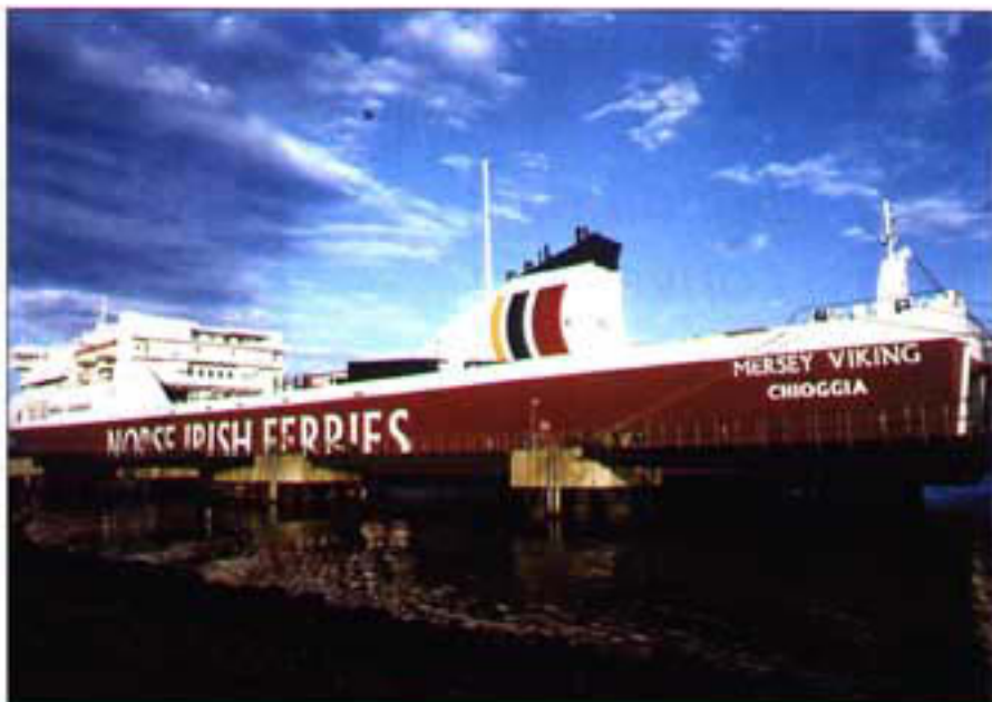
The 8000dwt Mersey Viking is another refined ro-ro ferry from the Visentini shipyard in Italy. A sister ship is scheduled for delivery this month.
